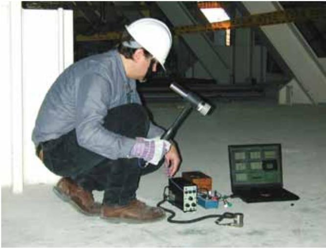
Fig. 1: During an impulse response test, the computer measures the signals produced by a load cell in the hammer and a motion sensor
