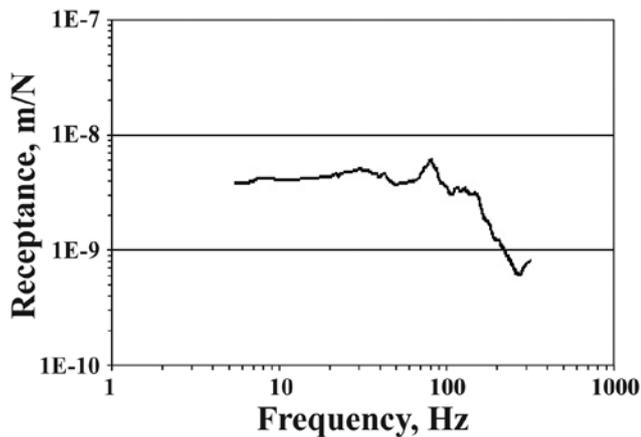
Fig. 2: A typical slab-on-ground receptance spectrum with a peak at 80 Hz that indicates a resonance frequency (1 m/N = 175 in./lb)
