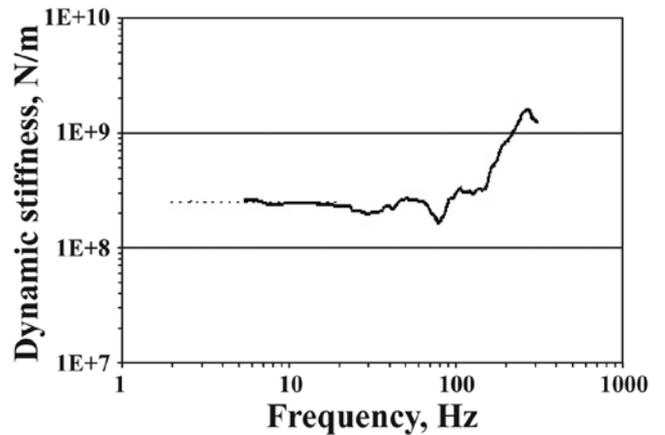
Fig. 3: The dynamic stiffness spectrum for the measurements shown in Fig. 2 is the inverse of the receptance spectrum. The dashed line is the static stiffness of the slab-foundation system. The resonance at 80 Hz now appears as a dip (1 N/m = 0.00571 lb/in.)
