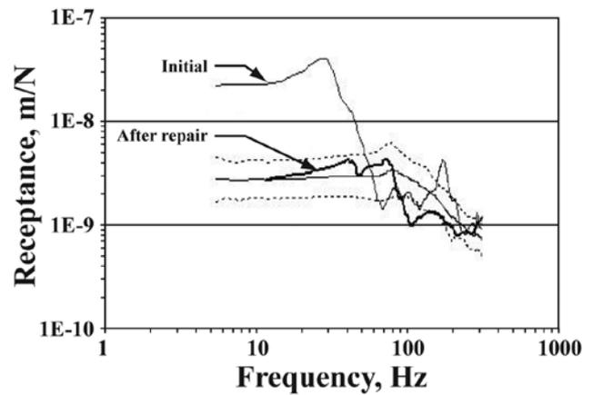
Fig. 8: Measured receptance spectra at the softest location before and after grout injection compared with the log mean and one-sigma limits for response of a normally supported slab (1 m/N = 175 in./lb)
