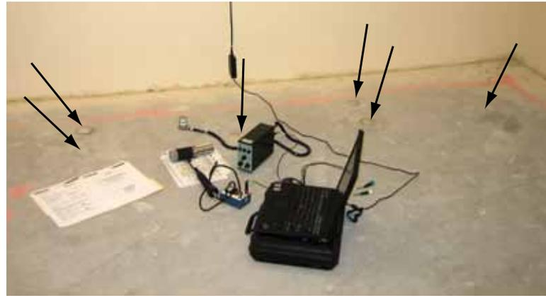
Fig. 7: Test setup at repaired area. Arrows indicate the plugged injection sites
