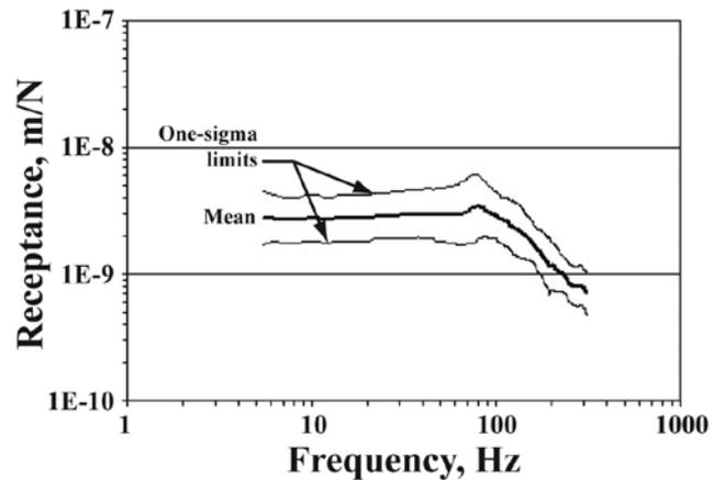
Fig. 5: The log mean receptance for the 22 locations shown in Fig. 4 and log mean  $\pm 1$  log standard deviation or one-sigma limits (1 m/N = 175 in./lb)
