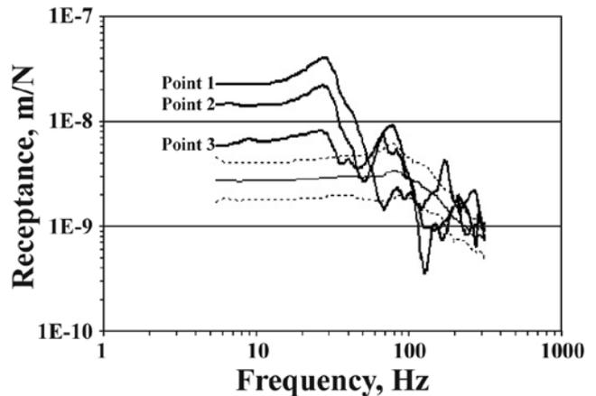
Fig. 6: Receptance spectra measured at three locations over a void, compared with the log mean and one-sigma limits of a normally supported slab (1 m/N = 175 in./lb)
