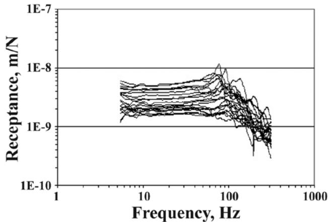
Fig. 4: Receptance spectra measured at 22 locations on a 150 mm (6 in.) thick slab-on-ground (1 m/N = 175 in./lb)
