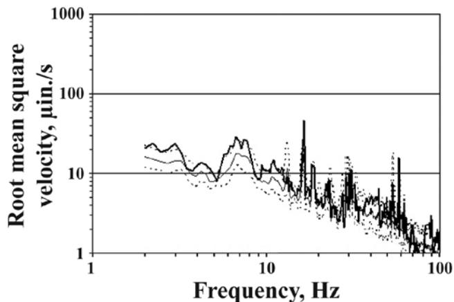
**Fig. 9: Ambient velocity spectrum (heavy line) at the softest location after grout injection measured with the facility in operation. The log mean (light, solid line) and one-sigma limits (light, dashed lines) for ambient vibration of a normally supported slab are shown for comparison (1  $\mu\text{in./second} = 25.4 \text{ nm/second}$ )**
