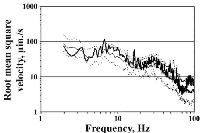
**Fig. 10: Footfall velocity spectrum (heavy line) at the softest location after grout injection. The log mean (light, solid line) and one-sigma limits (light, dashed lines) for ambient vibration of a normally supported slab are shown for comparison (1  $\mu\text{in./second} = 25.4 \text{ nm/second}$ )**
