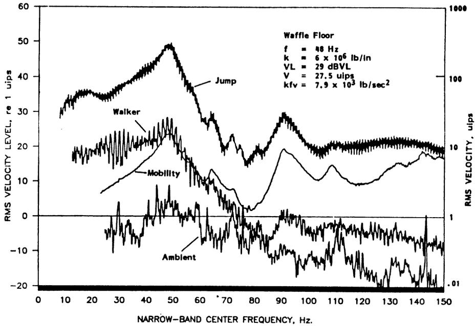
Figure 4. Vibration data measured on waffle floor.
