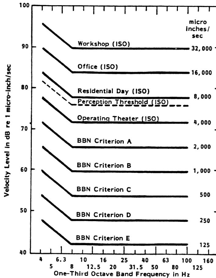
**Figure 1. Floor vibration criteria for equipment used in the production of integrated circuits [Other curves represent criteria recommended by International Standards Organization (ISO)]**
