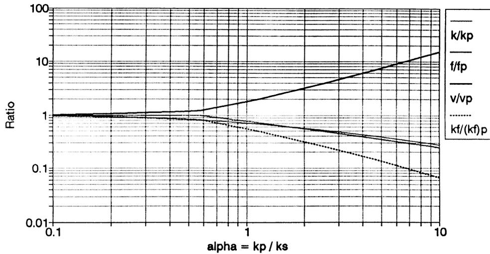
Figure 3. Dimensionless parameters for midpoint properties of multibay floor supported on springs.
