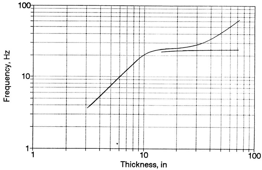
Figure 2. Frequency vs thickness for multibay floor supported on springs.
