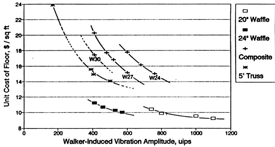
Figure 6. Comparison of the unit costs of several structural schemes as a function of walker-induced floor vibration performance.
