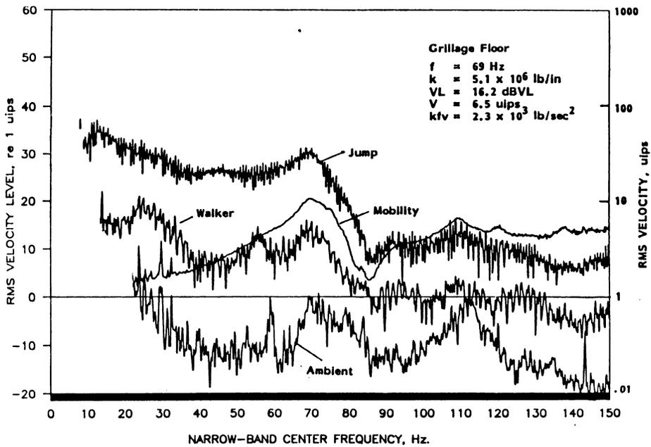
Figure 5. Vibration data measured on grillage floor.
