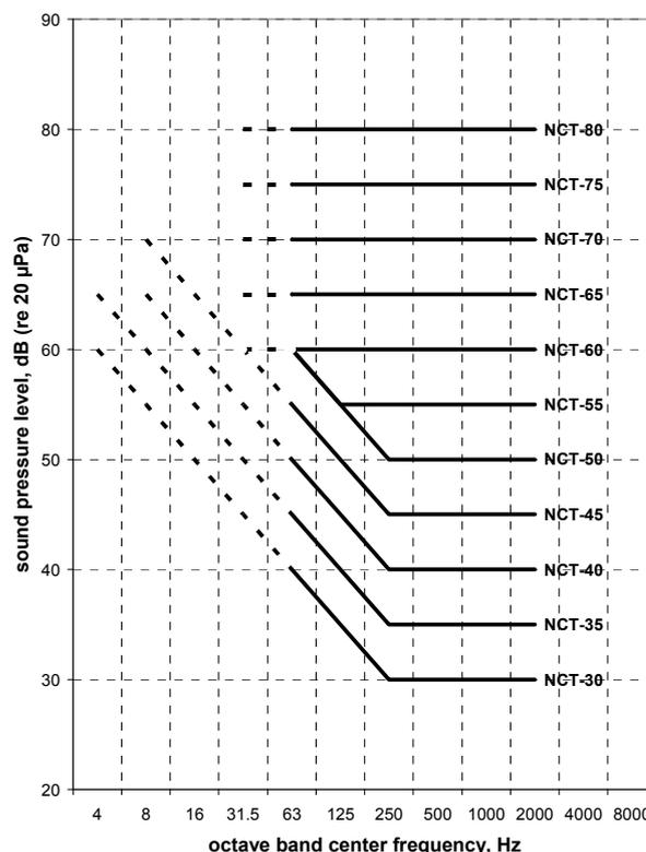
Fig.9 Generic noise criterion curves developed from the data analyzed.
