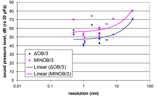
Fig.3 Representative noise sensitivity of several SEMs versus maximum rated resolution (various manufacturers and models).
