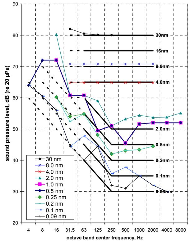
Fig.8 Lower boundaries of all data for various resolutions and generic noise criterion curves developed from the data analyzed.
