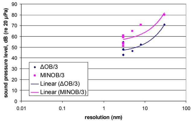
Fig.4 Representative noise sensitivity of several SEMs versus maximum rated resolution (one manufacturer, various models).
