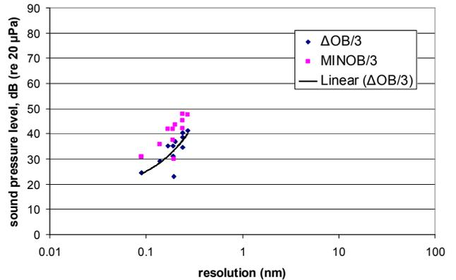
Fig.5 Representative noise sensitivity of several TEMs versus maximum rated resolution (various manufacturers and models).
