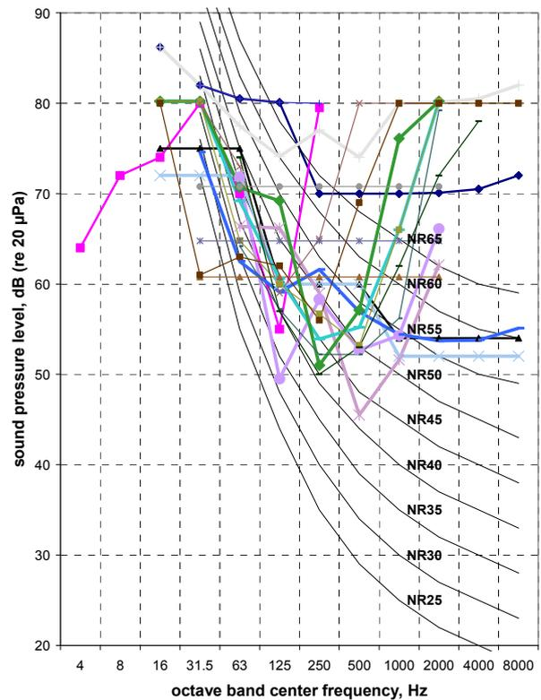
Fig.1 Manufacturer’s noise specifications (reduced to octave bands when necessary) for 19 SEMs.
