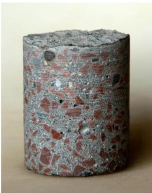
Figure 9: Core sample of 50mm concrete topping slab installed for Case 5 showing high-strength aggregate (brown).
